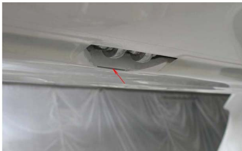
Fig. A: Inspection area: Trim tab control horn attachment point (Seen from underneath the stabilator)
