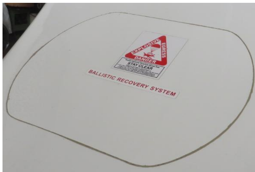
Fig. 5 – Sample view of warning label provided by BRS
