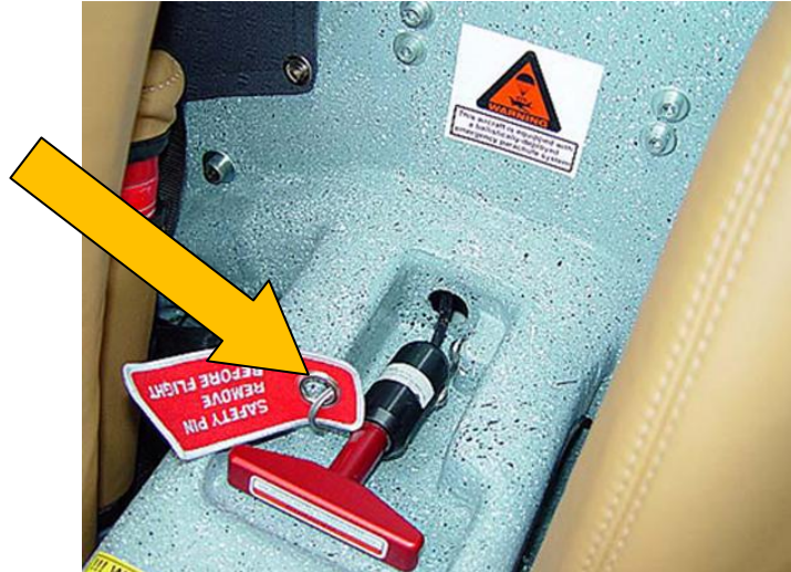
Fig. 1 – Sample view of BRS activation handle in a CTLS with locking pin inserted – other systems and aircraft models comparable.
